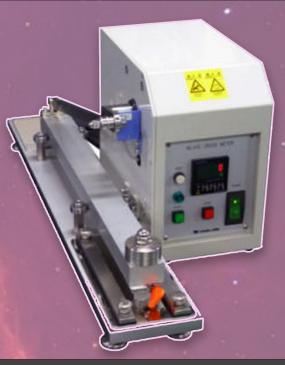
This tester is used to evaluate the color fastness of textile products, leather, rubber, and plastic against abrasion.
